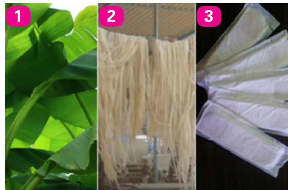
Figure 3: Picture showing a manufacturing process from banana tree (left) to a bio-degradable menstrual product (right).
